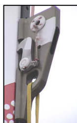
013080 - Headboard car with lashing on a 80 mm sheave for 2:1 halyard & lasheye for the main
