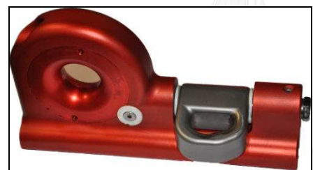
013070 - Headboard car with lashing on a 80 mm sheave for 2:1 halyard & articulated lasheye for the main
