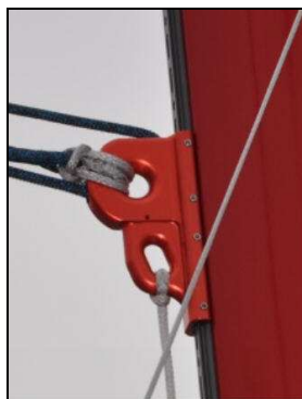
013080 - Headboard car with lashing on a 80 mm sheave for 2:1 halyard & lasheye for the main
