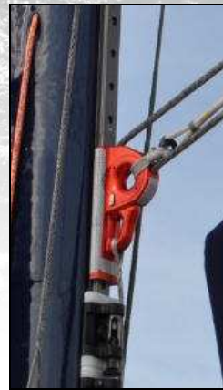
Headboard car with lashing on a 65 mm sheave for 2:1 halyard & lasheye for the main
