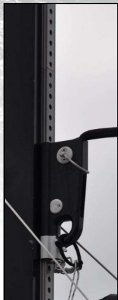
Headboard car with central hook, 70mm sheave & lashing for 2:1 halyard
